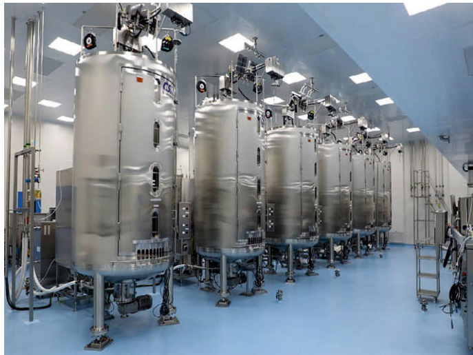
Covishield vaccine manufacturing facility using six single-use 4KL bioreactors at Manjari facility.
